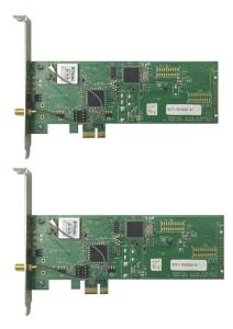
The Masterclock PCIe-GPS card receives reference time from atomic clocks orbiting in GPS (Global Positioning System) satellites to provide the most accurate time and date information. When locked to GPS (and the PCIe), your PC accuracy is ±2 milliseconds with reference to the source. High-stability oscillator options increase holdover accuracy to up to ±250ms/year.
